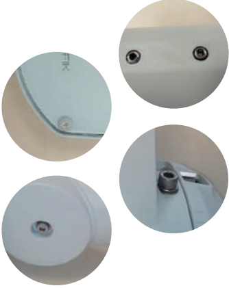
Pictures from a salt chamber after 1440 hours of tests.
